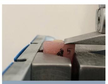
**Figure 1.** The SBS test SBS, shear bond strength
