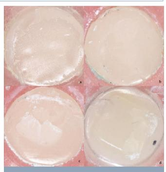
**Figure 3.** Stereomicroscope images of ceramic specimens RARI score 0 (a); RARI score 1 (b); RARI score 2 (c); RARI score 3 (d) RARI, resin attachment remnant index
