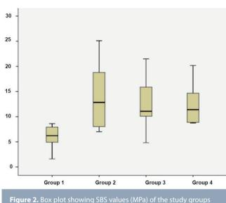
Figure 2. Box plot showing SBS values (MPa) of the study groups SBS, shear bond strength
