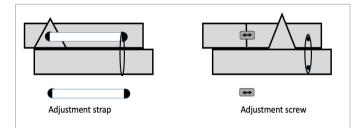
**Figure 1**. The illustration of the traction type of MAD (left) and the fin coupling type of MAD (right). The traction type of the appliance is adjusted by different lengths of the straps. The fin coupling type of device is adjusted using a screw in the upper jaw, which pushes the lower jaw forward with the help of a wing.
